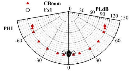
Figure5 Comparison of loudness levels for ground sonic boom signatures (Ma=1.23)
