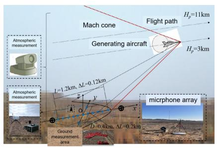
Figure 1 In-flight test method
