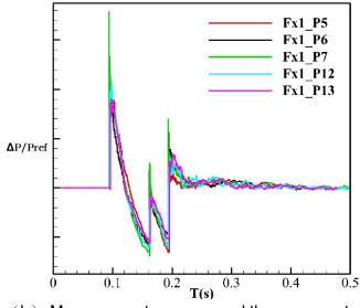
(b) Measurement array around the array center Figure 3 Measured sonic boom signatures
