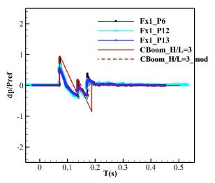
Figure 4 Comparison of over-pressure signatures for ground sonic boom (Ma=1.23)
