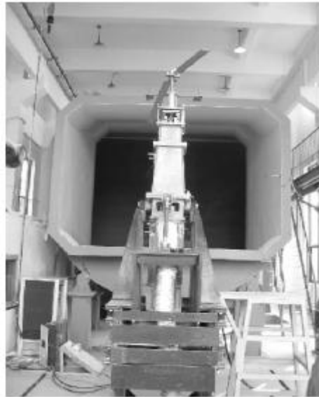
Figure 14 – Position of model rotor on rotor test rig during experiment [8] .
