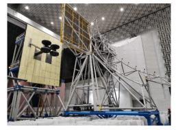
Fig.19 Landing gear noise test in FL-10 WT
