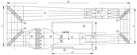
1.-open jet test section; 2.-collector; 3.first diffusor section; 4.-first corner; 5.-second corner; 6.-powe section 7.-second diffusor section; 8.-third
