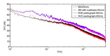
Fig.23 Noise spectrum w/o pantograph at 65m/s
