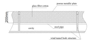
Fig.5 Outside acoustic treatment of wind tunnel
