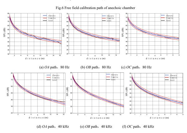
Fig.7 Sound pressure level attenuation curve of OA, OB, OC calibration path<sup>[12]</sup>
