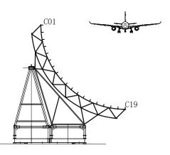
Fig 12 1/4 polar arc array (front view)
