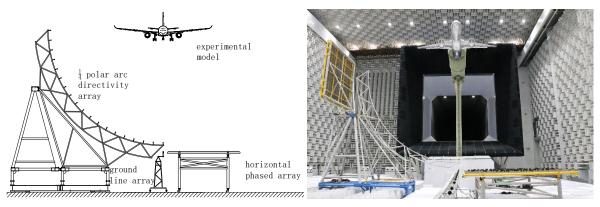
Fig 8 Array lay out for the scaled a/c model noise experiment
