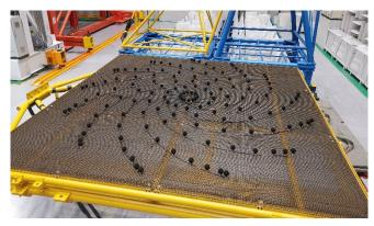
Fig 11 Vertical phased array (ground commissioning)
