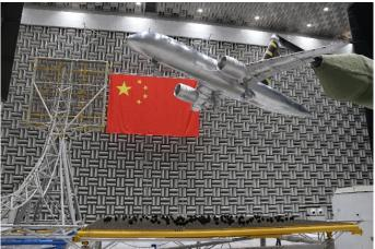
Fig.15 Airframe noise test in FL-10 WT
