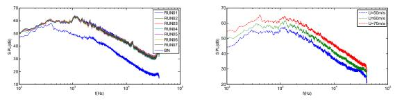
(a) Spectrum repeatability of takeoff configuration (b) Influence of wind speed on approach configuration spectrum Fig 16 Scaled aircraft noise test result
