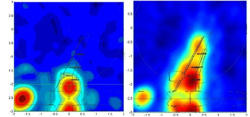
(a) Landing gear noise source localization result (b)Landing gear and high lift device noise source localization result Fig 17 Source localization result of scaled a/c
