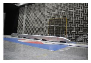
Fig 22 High speed train noise test in FL-10 WT
