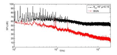
Fig.25 Helicopter noise test result in FL-10 WT
