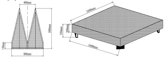
Fig.4 Sketch of acoustic panel
