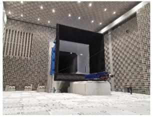
Fig.2 Anechoic chamber of FL-10 wind tunnel
