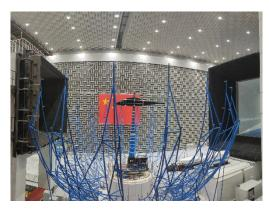
Fig 24 Helicopter noise experiment in FL-10 wind tunnel
