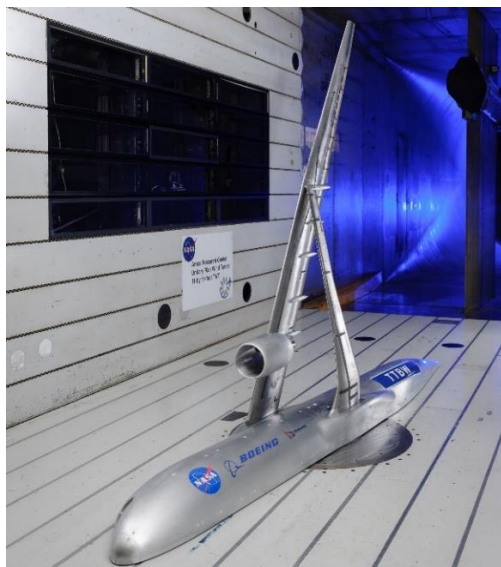
Figure 8. 9.0% Scale High-Speed Buffet Semi-Span Model in the NASA Ames 11ft Transonic Wind Tunnel
