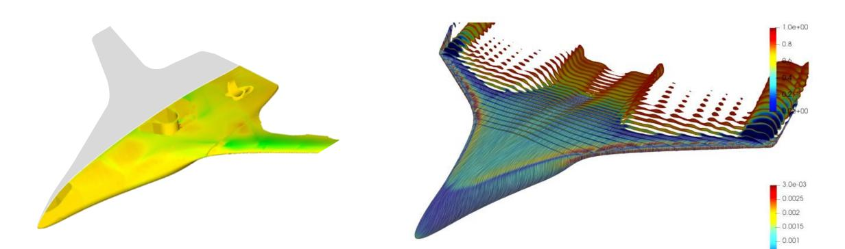
FEA Strength and deflections Flutter analysis CFD validation of Rn-corrected airfoil stack
