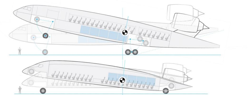
Thickness and chord are reduced with a Single Deck
