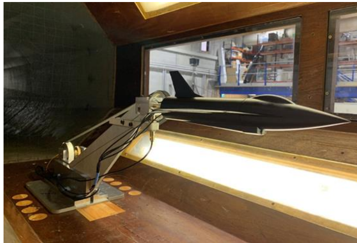
Figure 3 - The SDM tunnel support system.
