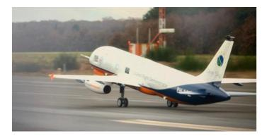
Figure 7 : Rotation Manoeuvers made with the SFD during the Taxi tests
