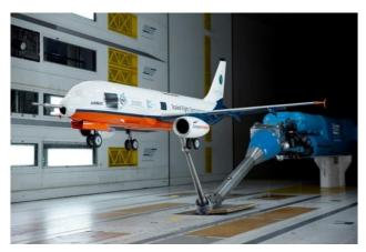
Figure 4 : Wind Tunnel Test installation of the SFD (DNW)
