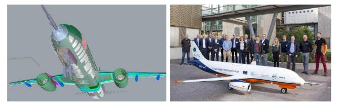
Figure 2 : Detail digital mock-up of the SFD (left) and integrated SFD at the end of the development (right)
