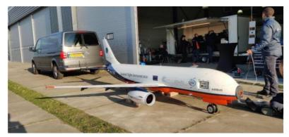
Figure 6 : First ground runs test of the SFD at Breda Airport
