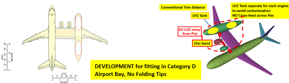
Figure 8 - Twin-Fuselage Layout using LH2, Central Engines
