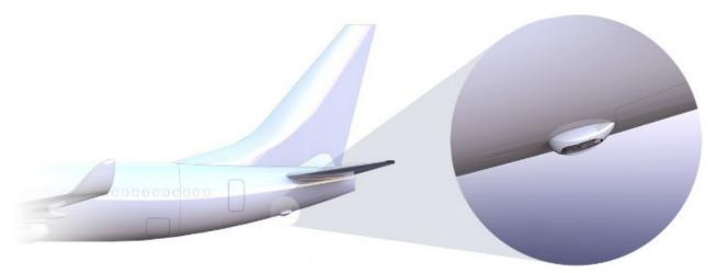
Figure 1 – Schematics of ORCA Installation on an airliner [3]
