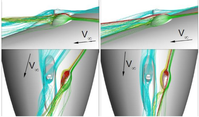
Figure 2 – Indicative flow topologies showing the radome wake characteristics with negative AoS
