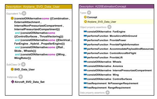
Figure 8 – The definition of the *Airplane\_SVD\_Data\_User* class (left) and the *A220 Estimation Concept* individual with inferred information highlighted in yellow background (right).
