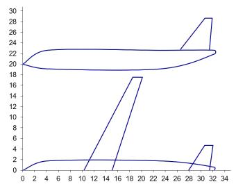
Figure 13 – The aircraft's initial geometrical layout (all dimensions are shown in meters) which has been obtained by inserting the SVD analysis values together with minor changes to the sweep angles of all lifting surfaces.
