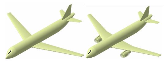
Figure 14 – The 3D geometry in *Robust Aircraft Parametric Interactive Design* (RAPID); initial geometry obtained by inserting the SVD analysis values (left) and the updated geometry with a kink wing (right).
