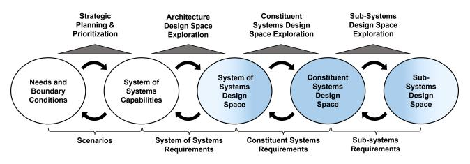
Figure 1 – An outline of the holistic *System-of-Systems* (SoS) design process, which has been adapted from [2]. The highlighted circles show the area that this work is addressing.
