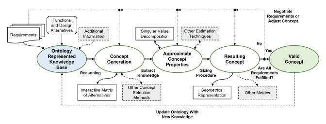
Figure 3 – An illustration of the proposed method and the overall workflow to generate valid concepts from an ontology description.
