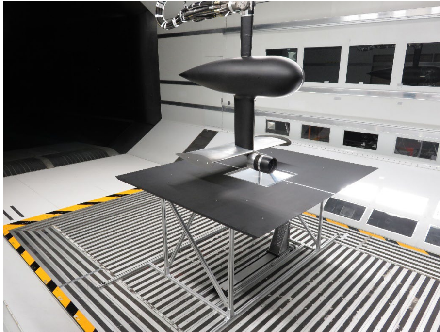
Figure 17 – TRUflow wind tunnel model installed in the RUAG LWTE test section, with thrust reverser in the deployed configuration
