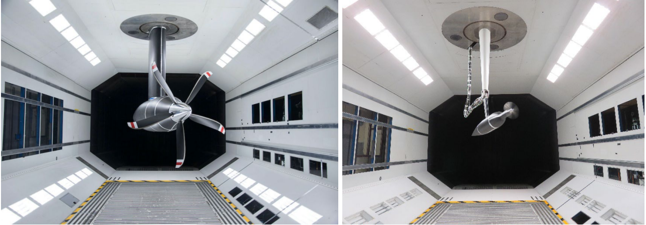
Figure 3 – Isolated full- and model-scale propeller test for Textron McCauley
