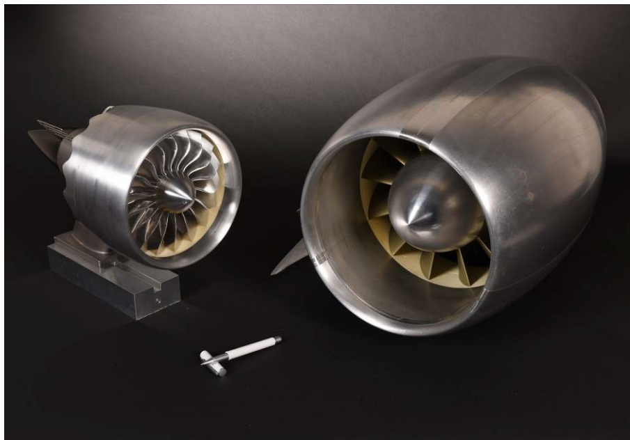
Figure 10 – Mini-turbofan simulator (left) with pylon integrated in the motor case (based on MR09). On the right: Turbofan simulator for ESICAPIA, based on an MG20 motor.
