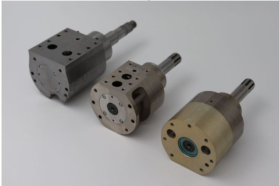
Figure 9 – Three hydraulic motors of the same type with different case and inlet/outlet interfaces
