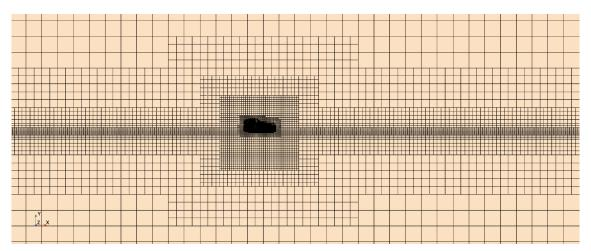
Figure 3 – Domain shape and mesh. It is visible a denser mesh at the fluid interface and in two size box centred in the hull.
