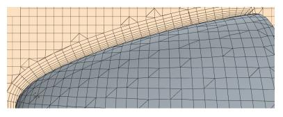
Figure 4 – Prism Layers
