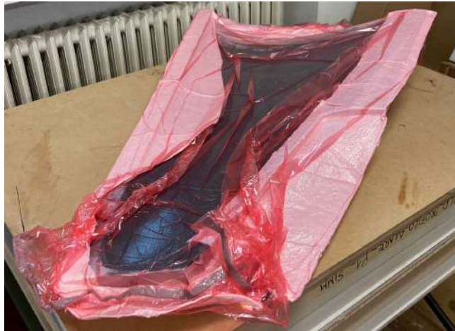
Figure 22 – Laminated skin in the vacuum bag
