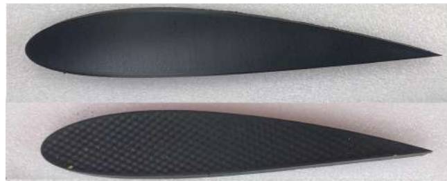
Figure 16 – Comparison between the mould after the first (top) and the last (bottom) lamination process
