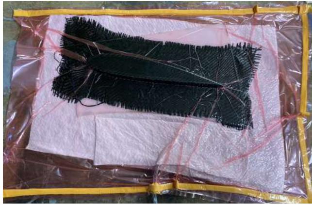
Figure 11 – Laminate is put in vacuum bag
