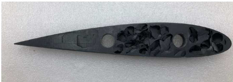
Figure 12 – Final result of the additive mould (7% filling)
