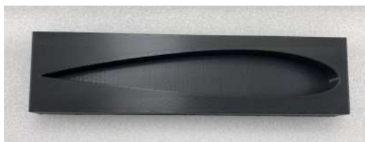
(a) Model for gelcoat and fibreglass mould
