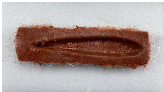
Figure 9 – Lamination with fibreglass of mould
