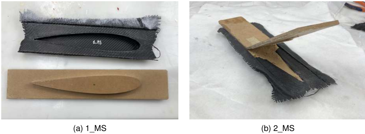
Figure 17 – MDF with draft angle results
