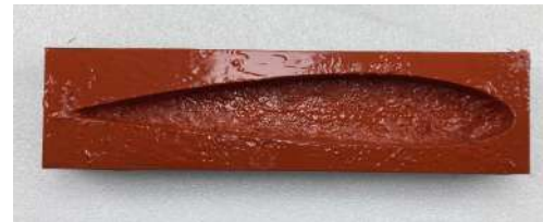
(b) Layers of gelcoat applied on model
