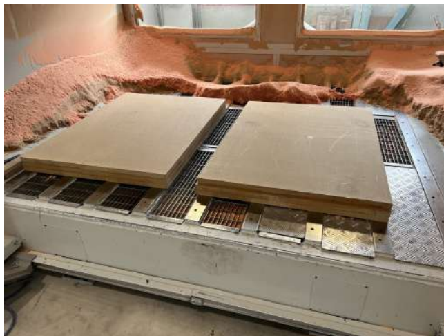
Figure 24 – MDF sheet ready to be milled
