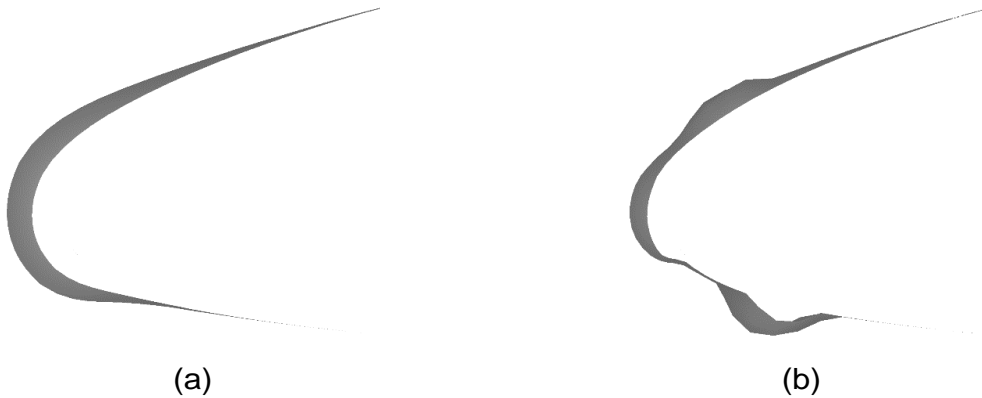
Figure 9 – Ice Shape formation for (a) Rime (b) Glaze Ice type using ICE3D.
