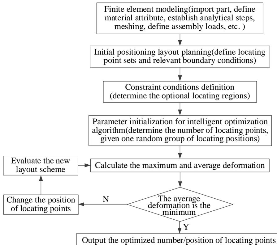
Figure 2 – Solution method for determining locating points for parts with a weak rigidity
