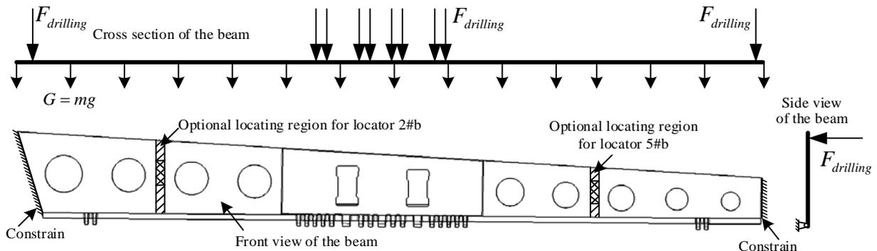
Figure 7 – Assembly loads and constraints of the inner beam
