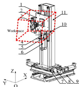
1. Guiding rail; 2. Connecting plate; 3. End locating effector ; 4. Connecting flange; 5. Shaft coupling; 6. Servo motor;
