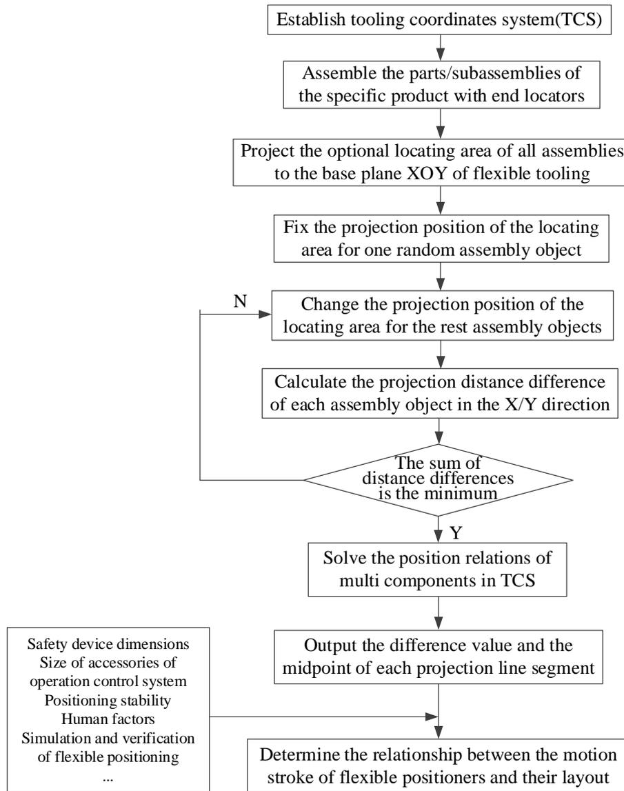
Figure 1 – Motion stroke and layout optimization process of flexible locators
