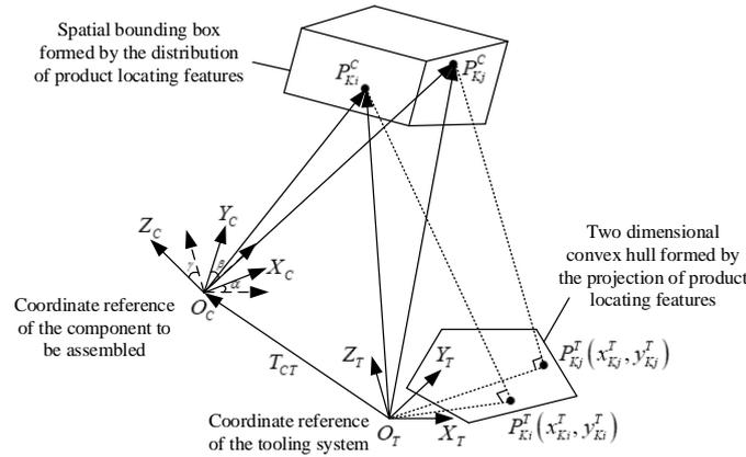
Figure 3 – Transformation from spatial bounding box to two-dimensional convex hull by projection
