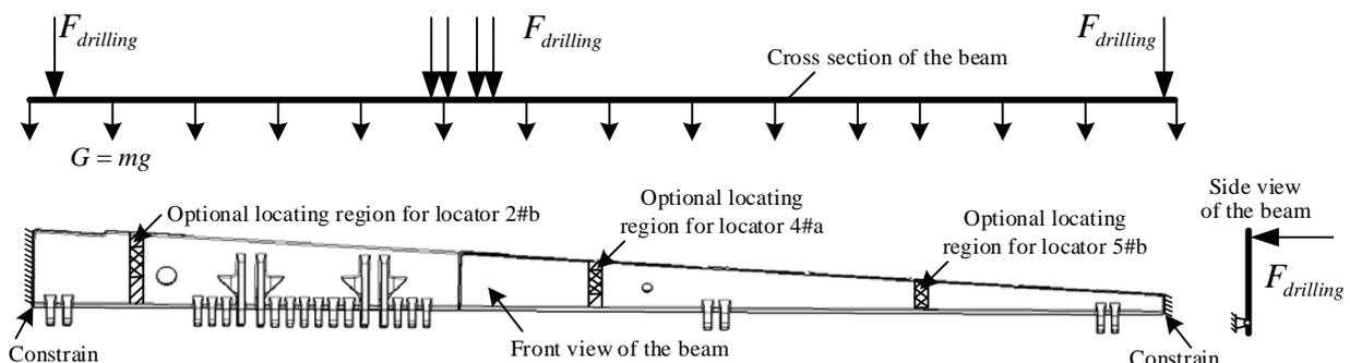
Figure 8 – Assembly loads and constraints of the outer beam
