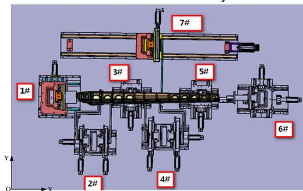
Figure 9 – Layout relationship among the locating units of the flexible tooling system
