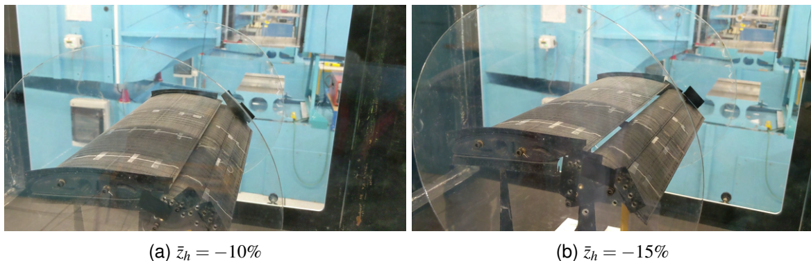
Figure 10 – Double-slotted flap model at 30^\circ flap setting and two hinge positions
