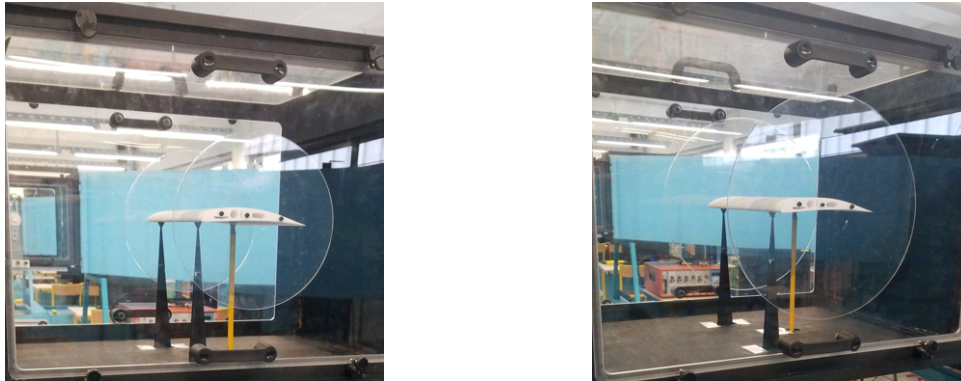
(a) Closed section with 1.5c diameter end plates (b) Closed section with 2.0c diameter end plates
