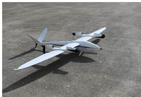
Figure 13 - The Emergency Service Drone with integrated MACS aerial camera system for real-time mapping applications
