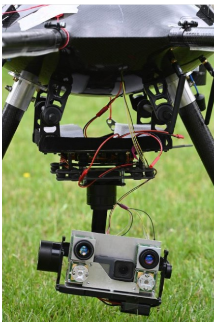
Figure 19 - Horizontal and vertical LIDAR installed on gimbal, together with a small camera in the center
