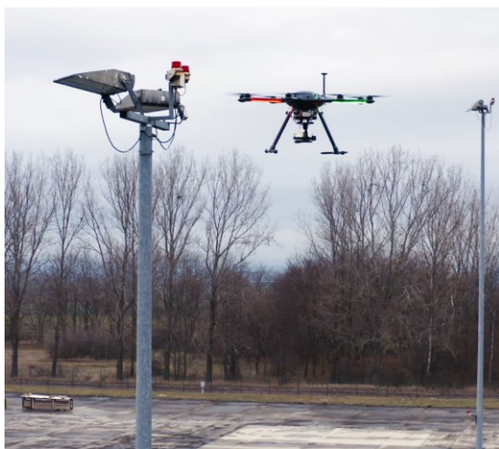
Figure 21: Detection of a lamp post with LIDAR sensors
