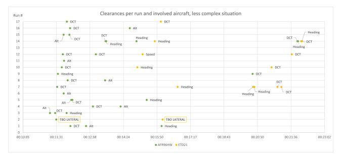
Figure 5 – Clearances for the less complex conflict, scenario 6. Clearances given around minutes 11 to 12 shows initial clearances to solve the conflict. Most clearances from minute 13 to 17 are adjustments to ensure separation, while clearances after minute 19 are given to resume own navigation to original route when the conflict is over.
