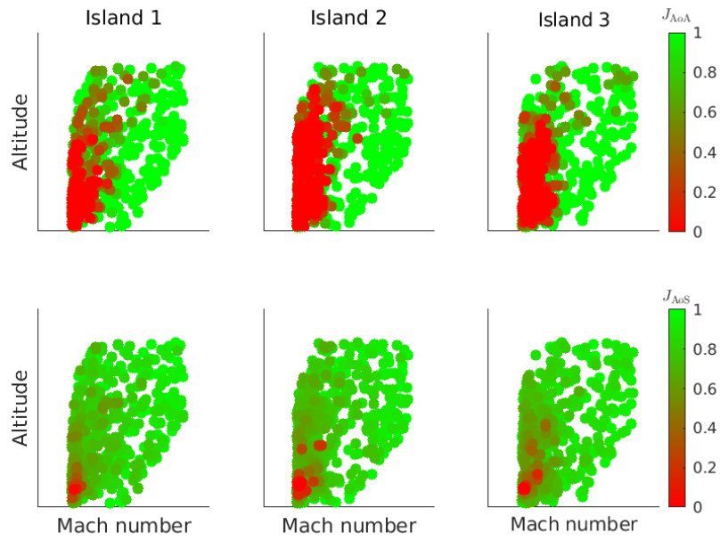
Figure 10 – Objective values after two migrations plotted inside flight envelope for the three islands based on NSGA2 algorithm evolution.
