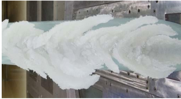
Figure 1 – H.T. critical icing shape
