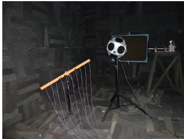
Figure 1 – Acoustically treated test chamber, with the omnidirectional sound source and one of the five microphone paths to test the chamber acoustic performance.
