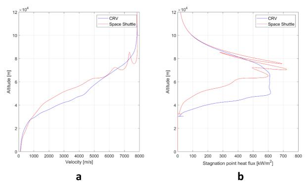
Figure 7 a-b – Comparison between Shuttle-like GL re-entry trajectory and CRV admissible re-entry trajectory: Re-entry trajectory vs. altitude (a); Stagnation point heat flux vs. altitude (b).
