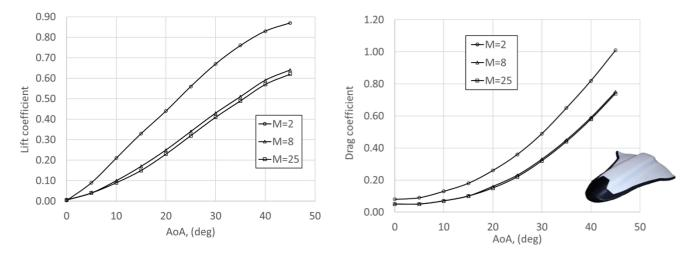
Figure 5 - CRV high-Mach numbers clean configuration aerodynamics.
