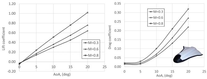
Figure 6 – CRV low-Mach numbers clean configuration aerodynamics.
