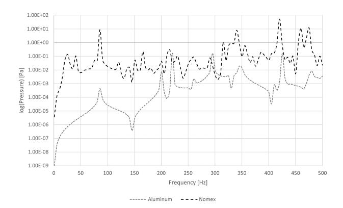
Figure 4 – The frequency response of the cylindrical cavity coupled to a cylindrical shell for Point B, the results show the comparison between an honeycomb material, similar to Nomex, and aluminum
