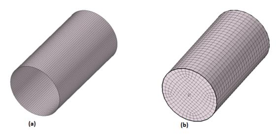
Figure 2 – The FEM geometry on which the natural mode are extracted. (a) Shell structure. (b) Cylindrical fluid cavity.
