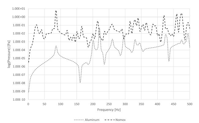
Figure 3 – The frequency response of the cylindrical cavity coupled to a cylindrical shell for Point A, the results show the comparison between an honeycomb material, similar to Nomex, and aluminum.
