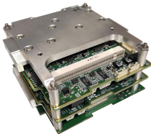
Figure 2 - Photograph of SpaceCloud iX5-100 radiation-tolerant cloud computing solution.
