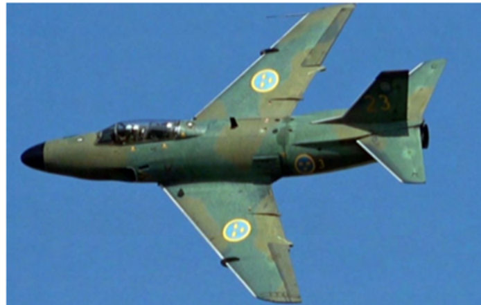
Figure 4 – The Saab 32 M 1 fighter, maiden flight 1952. Note the leading edge fence.
