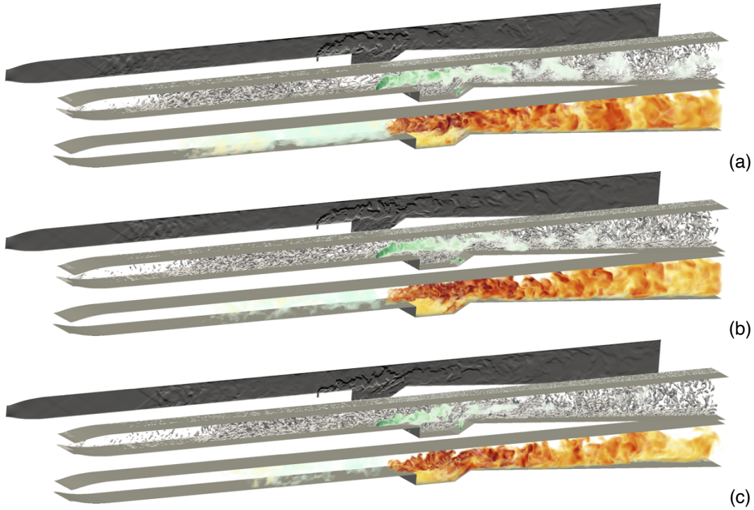
Figure 4. Perspective views of the flow in terms of the refraction index gradient, \nabla n , the 2 nd invariant of the velocity gradient, \lambda_2 , (gray) and the H 2 mass-fraction (green), and the temperature, T , (warm colors) for (a) Case F1, (b) Case F3 and (c) Case F5.
