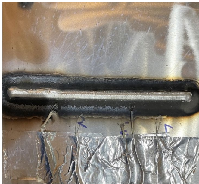
Figure 5 - Thermocouple placement relative to the centerline
