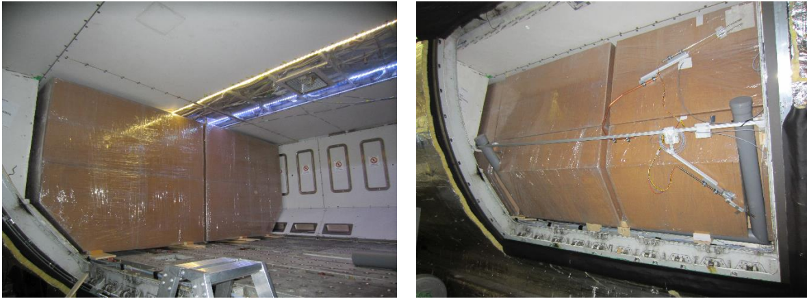
Figure 5: Containerized cargo hold during integration (left) and 100% loaded (right)
