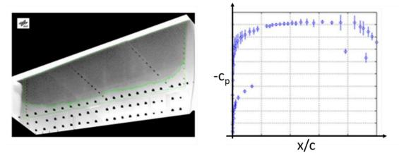
Figure 3 –IR data including a transition line (left, data from DLR) and pressure measurements including 95% confidence interval (right, data from AIRBUS).
