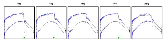
Figure 5 – Comparison of pressure coefficient from CFD calculations with flight test measurements.
