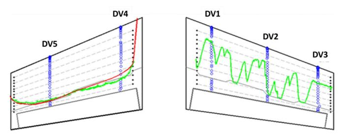
Figure 6 – Transition lines used for the CFD calculations based on flight-tested data, detected by DLR shown in green and some minor adjustments from Saab in red for the left wing panel.
