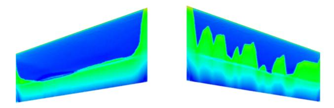
Figure 7 – Skin friction from CFD calculations based on transition line from flight test.
