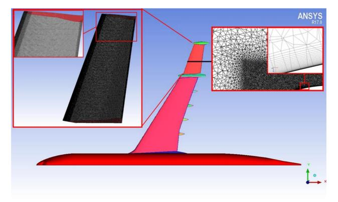
Figure 4 – Geometry provided by AIRBUS and parts of the mesh used for the CFD analysis.
