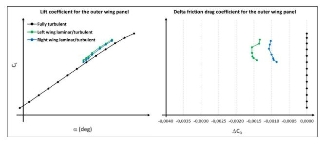
Figure 8 – Lift and delta frictional drag coefficients for the fully turbulent, left and right wing panel.
