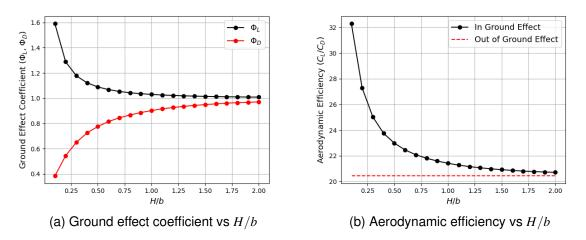
Figure 2 – Influence of ground effect coefficient and aerodynamic efficiency on ratio of distance from ground to wingspan (H/b) for the baseline wing
