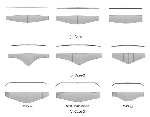
Figure 5 – Optimized planform shapes obtained from all the three cases. Left side shapes corresponds to best L/D ratio, right side shapes corresponds to best  $C_{L,h}$ , shapes in the middles corresponds to best compromise solution
