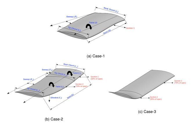
Figure 1 – Parametrization of the baseline wing with design variable definitions
