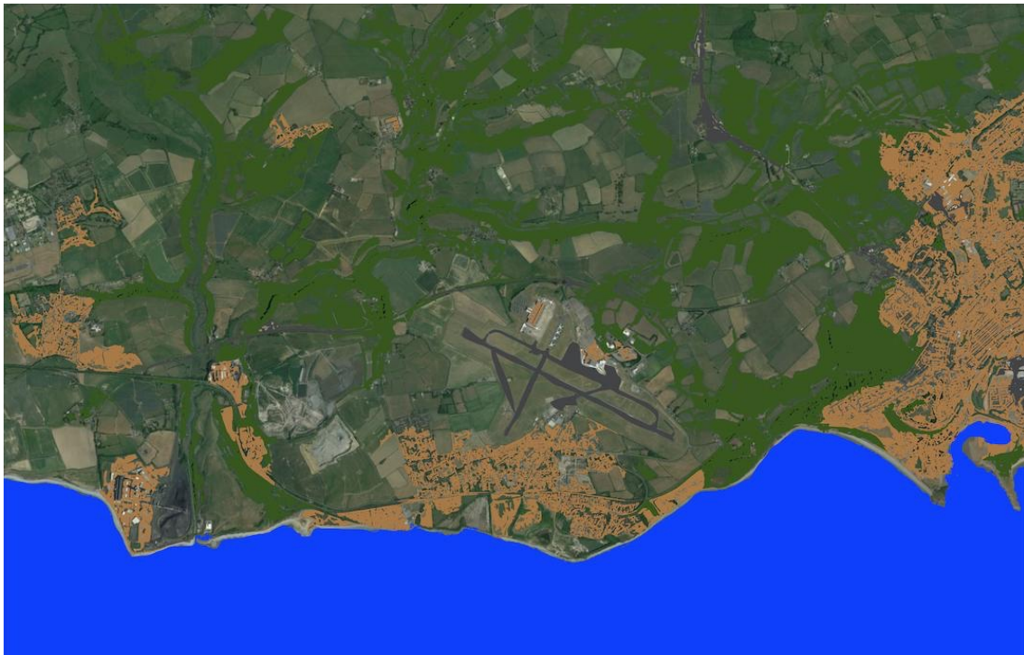
Figure 3 – Colour classification of terrain type (blue = water, light brown = built up area, dark green = trees, dark grey = road / tarmac, light green = grass and similar). The colours are automatically converted into a roughness length map for the terrain as per Table 1.
