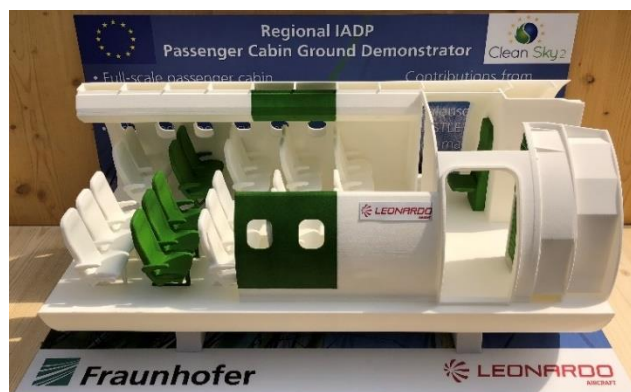
Figure 18: 3D printed model of the Passenger Cabin Ground Demonstrator
