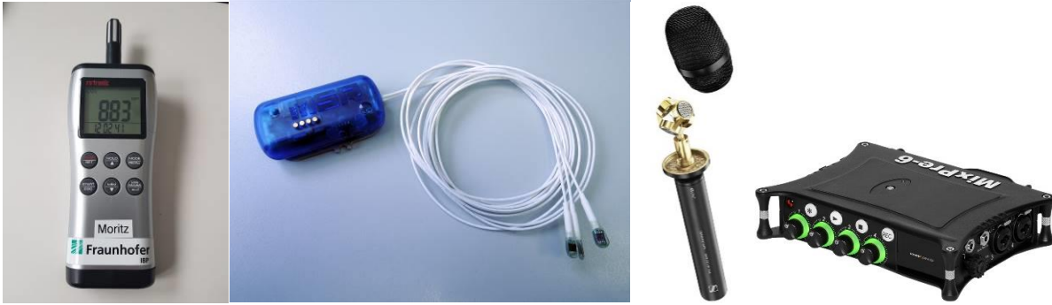
Figure 2: Measurement equipment. Left: CO 2 & RH, middle: temperatures and pressure, right: acoustics
