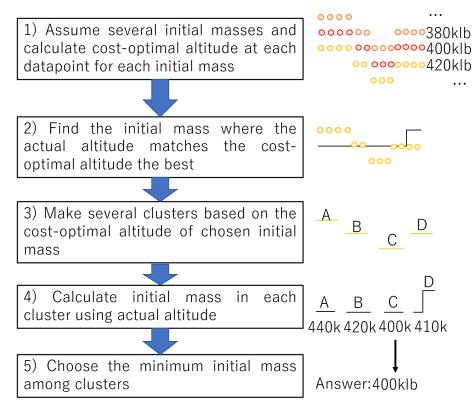
Figure 4 – Example of flight altitude and cost-optimal altitude of various mass.
