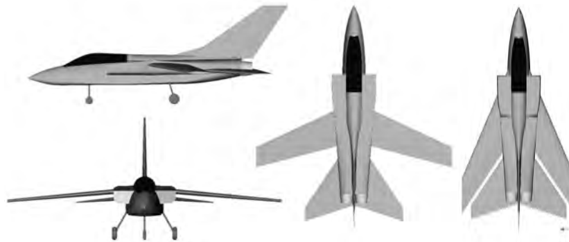
Figure 9 – Redesigned MRCA Tornado aircraft with 25° and 67° wing sweep
