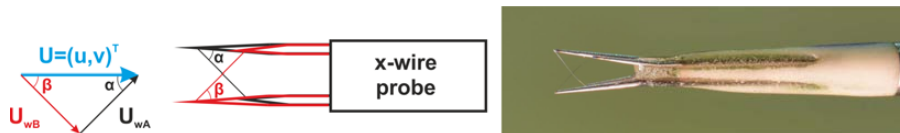
Figure 18 – X-type hot-wire probe.
