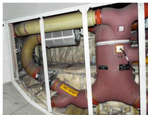
Figure 24: Example of a combined HEPA and carbon filter fitted to an A319
