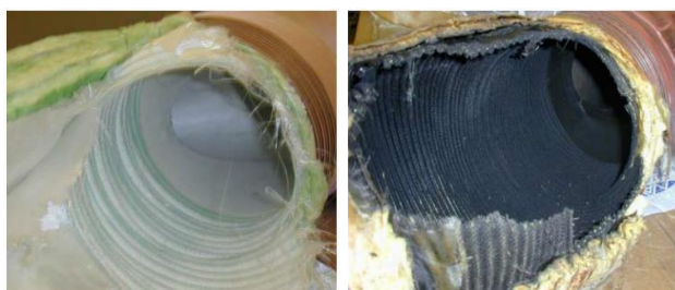
Figure 4: BAe 146 new ECS ducting (left) and used ducting (right)
