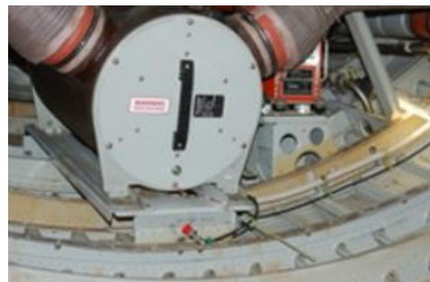
Figure 9: AirManager cabin air system installed in BAe 146
