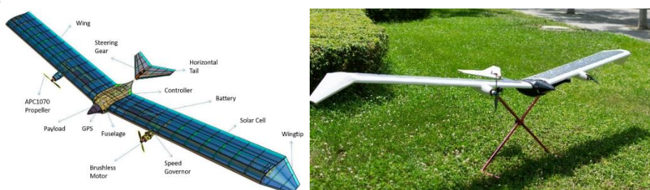
Figure 1 – The bionic hand-launched solar-powered UAV system MY-01.
