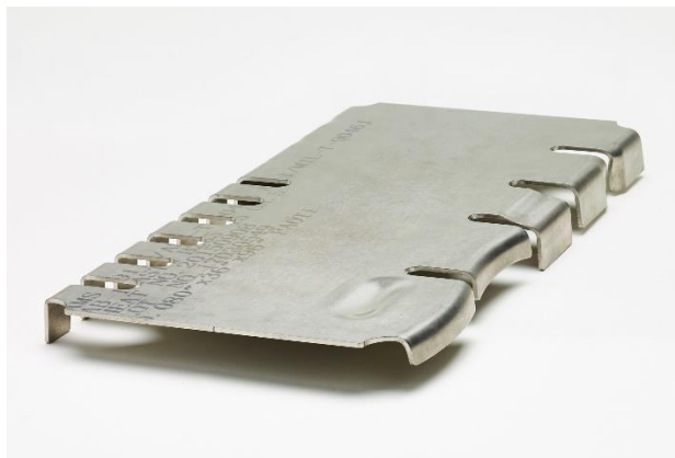
Figure 8 – General demonstrator designed with several features, like joggles, dents, various bend radius, shrink and stretch flanges, typical challenges in airframe part manufacturing.
