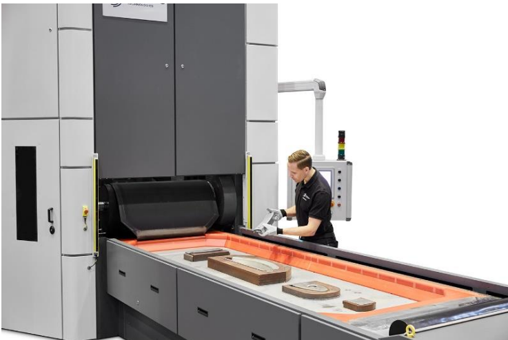
Figure 2 – Example of a Quintus fluid cell press cold forming operation, where several forming tools are loaded in a shuttling tray, then processed inside the pressure chamber, all tools at the same time in one and the same forming operation.
