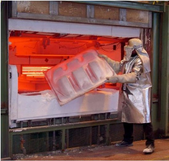
Figure 3 – Example of a traditional hot forming process, now challenged by a lower temperature high pressure process. Cycle times for hot forming are typically hours, producing one part at the time.
