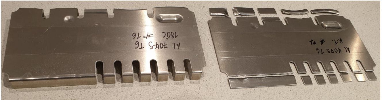
Figure 7 – Illustration of the difference in formability of Al 7075-T6, t=1.6\text{mm} , at ambient temperature and at 180^\circ\text{C} . A similar effect is visible also for Ti 6Al-4V and for Al 2024-T3.
