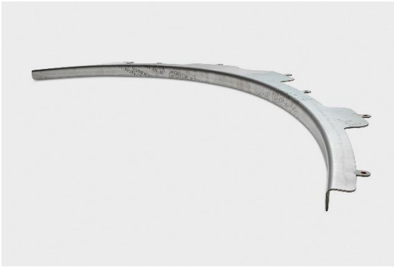
Figure 11 – The part could successfully be formed at a temperature of only 270°C, when combined with high pressure of 140 MPa.
