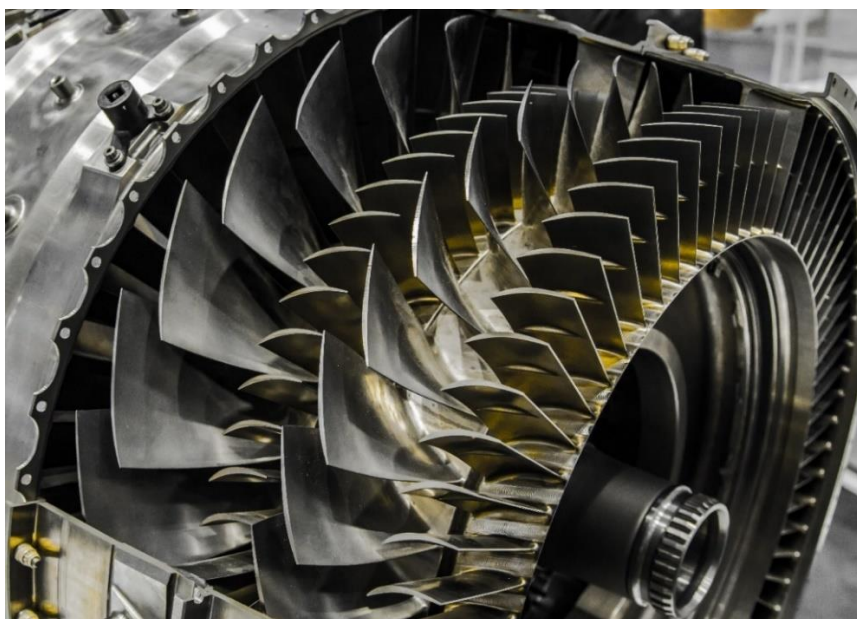
Figure 9: An aero engine is a complex piece of equipment with high fatigue loads and temperature variations
