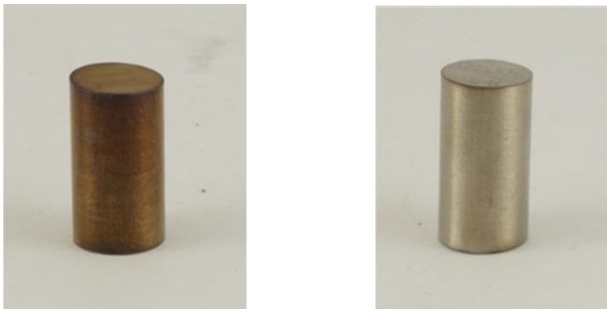
Figure 8: Alloy 718 bars treated with traditional hot isostatic pressing (left) and modern Quintus processing (right)
