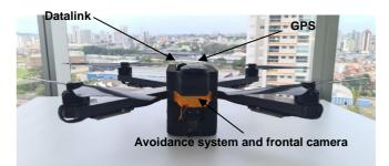
Figure 2 - BRV-03, Electric UAV prototype.
