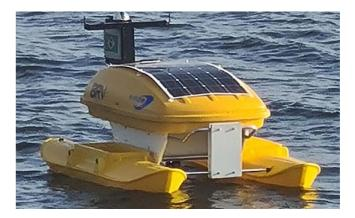
Figure 7 - USV boat prototype.
