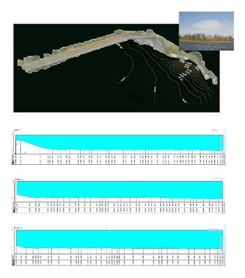
Figure 23 - Boat mission with the points collected by underwater sonar and a depth, graphics representation (topography).
