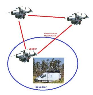
Figure 10 - Swarm drone coordination model by hierarchical coordination.
