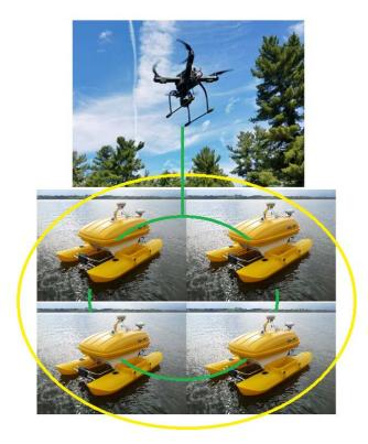
Figure 9 - Swarm architecture for mapping application (Squadron).
