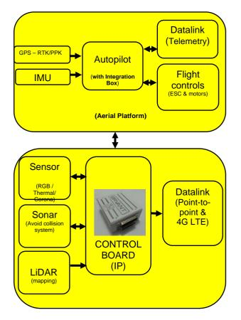
Figure 3 - The onboard equipment integration diagram.
