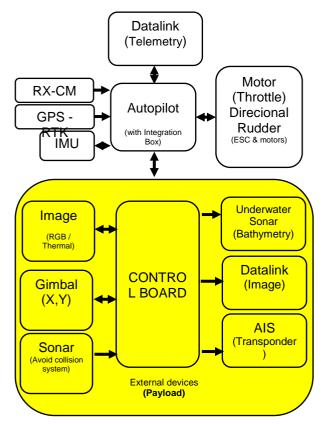
Figure 8 - Boat: The onboard equipment integration diagram.
