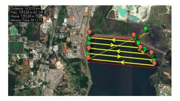
Figure 18 - Quadcopter or Boat, mission profile.
