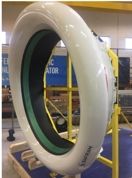
Figure 17 : Scale 1:1 short inlet nacelle demonstrator hardware
