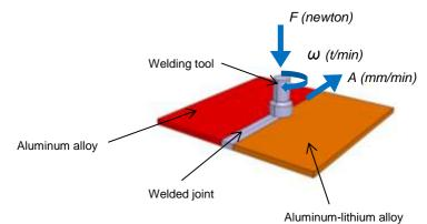
Figure 4 – Welding configuration.
