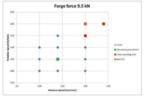
Figure 5 – Welding parameters.
