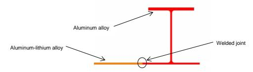
Figure 3 – Design configuration.
