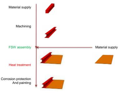
Figure 9 – Manufacturing process.
