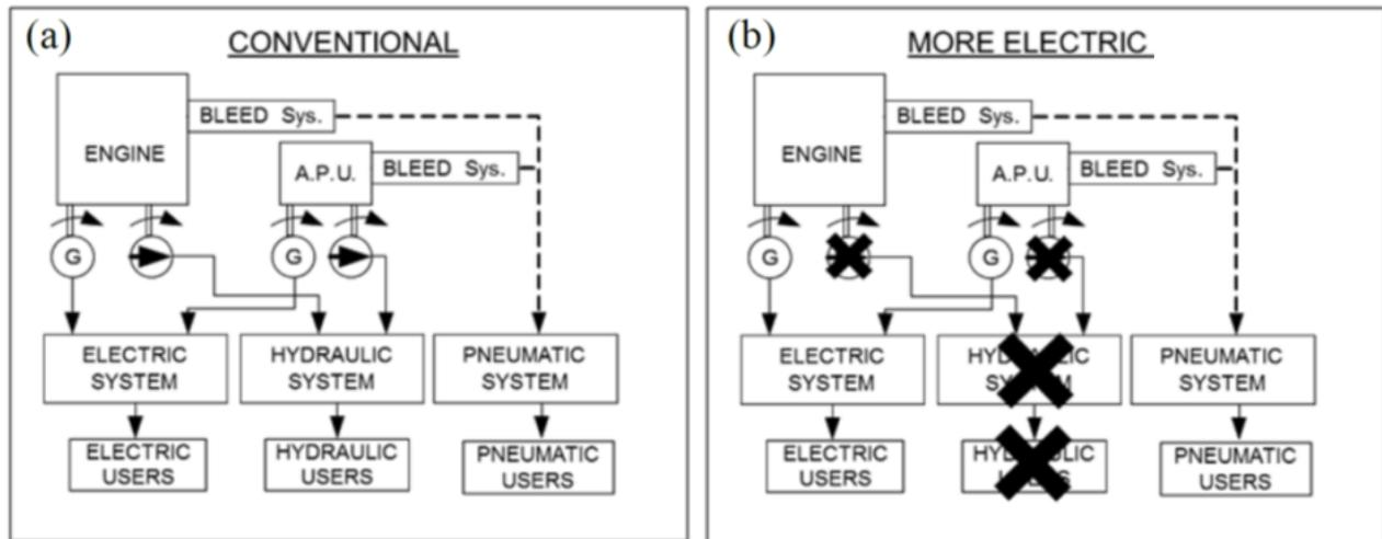
Figure 2 – Comparison between conventional and MEA architectures
