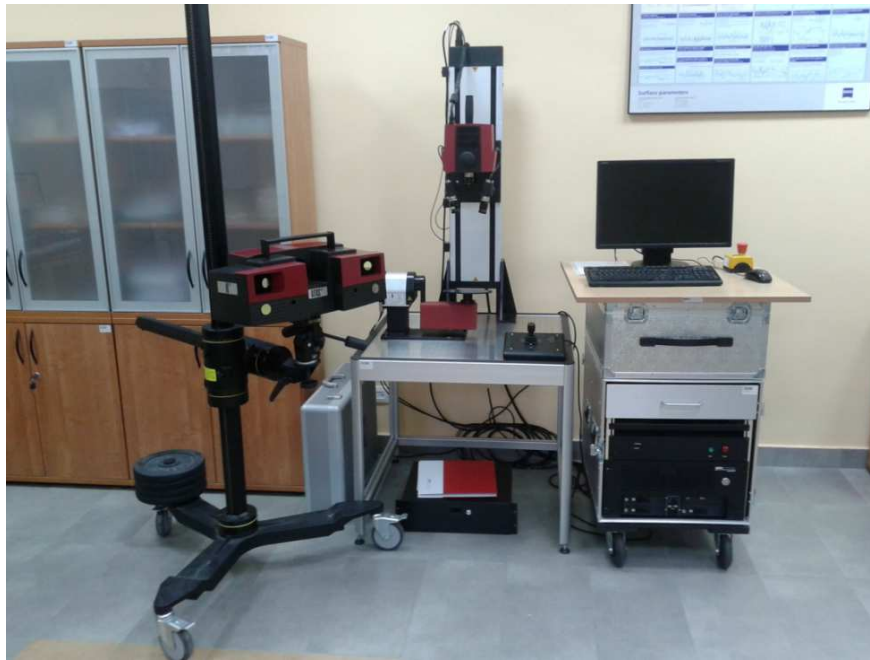
Figure 1 - ATOS II Triple Scan and ATOS Compact Scan optical measuring systems.
