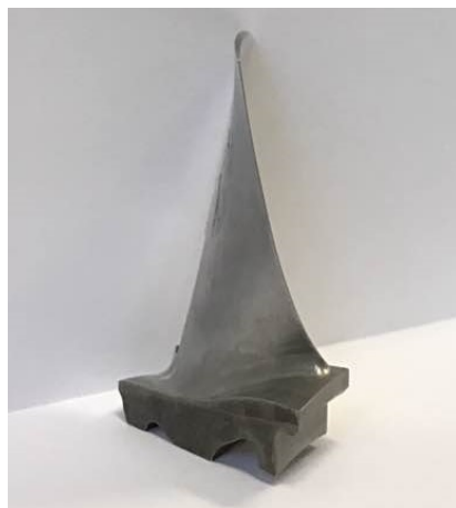
Figure 1 A compressor blade of turbine-shaft engine.
