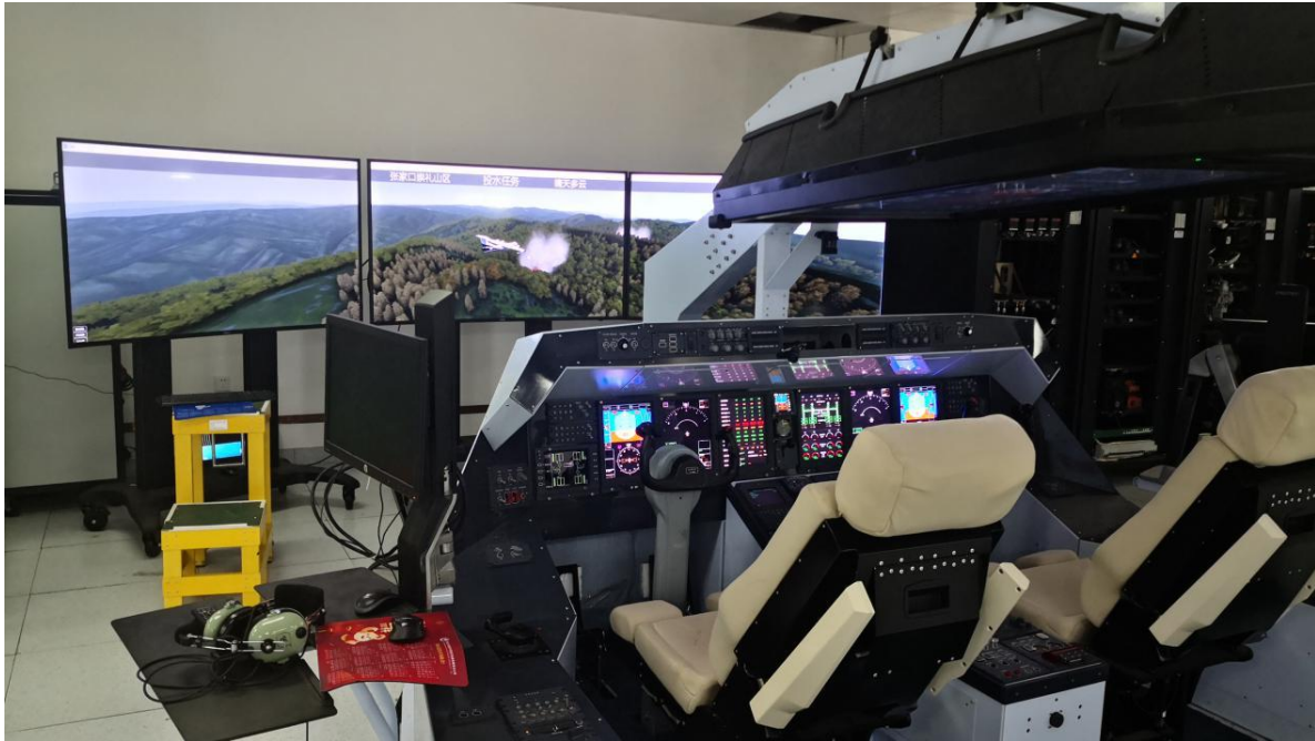
Figure 12 – Simulation effect of human-in-the-loop semi-physical fire extinguishing flight simulation system
