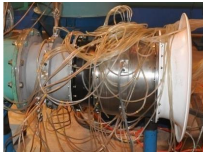
Figure 9 – Installation of the test rig and instrumentation pipes.
