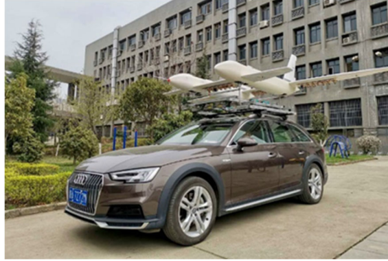
Figure 4 – Ground Vehicle-Based Testbed of the DEP Verification UAV
