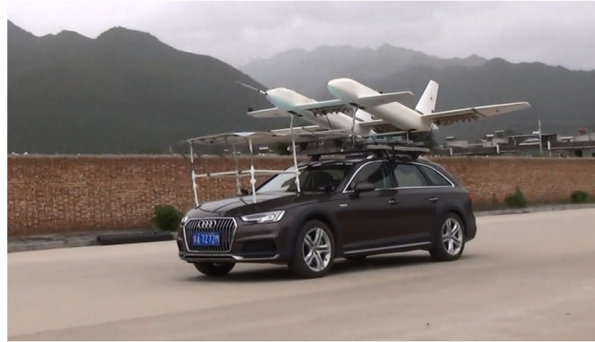
Figure 5 – Ground Vehicle-Based Testbed with Flow Divider
