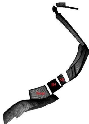
Figure 3 – Computation mesh of the compressor including the struts.
