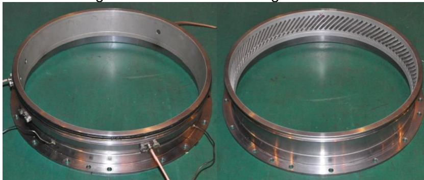
Figure 2 – The parts of solid wall (left) casing and casing treatment (right) of the first rotor.
