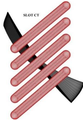
Figure 4 – Detailed grid of the skewed slot and first rotor.
