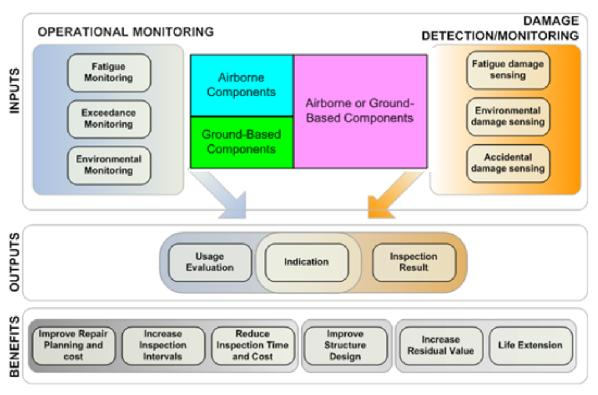
Figure 1 - Structural Health Monitoring following ARP 6461 [2]
