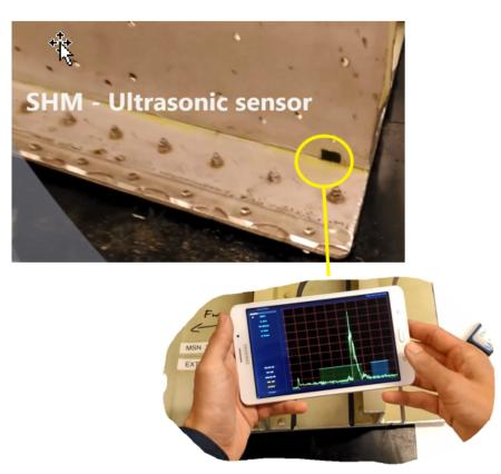
Figure 5 - Example of on-ground sensor interrogation
